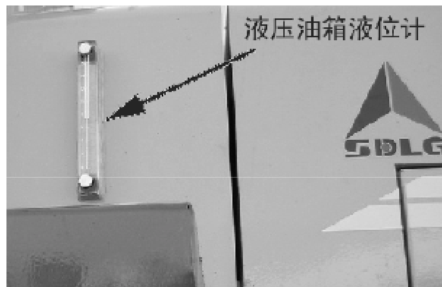
Hydraulic oil level gauge
