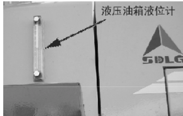
Hydraulic oil tank level gauge
