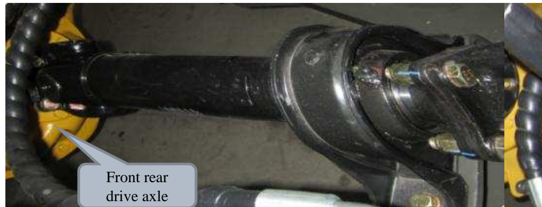
Front drive shaft: for connecting SDLG transmission with front drive axle
