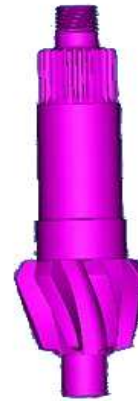
Front axle drive spiral bevel gear, left-handed
