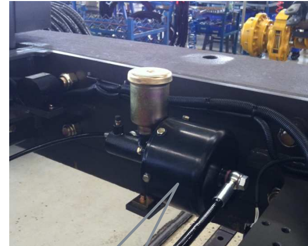
Rear booster pump position
