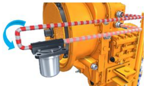
Fig. 2-14 Filtered Oil to Transmission Control
