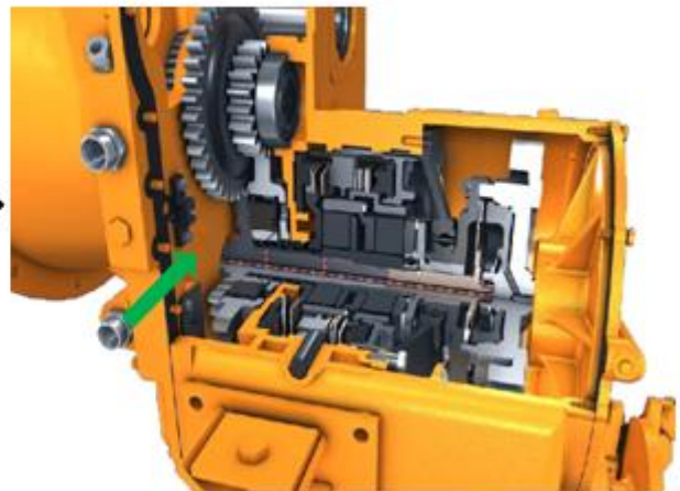
Fig. 2-20 Lubricating Oil Circuit in Transmission
