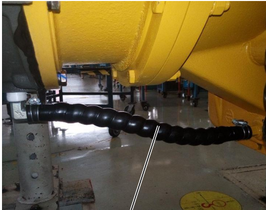
Fig. 4-25 1 Oil return pipe
