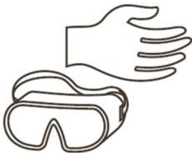
Fig. 11 When a risk of touching refrigerator is involved, do wear protective goggles and gloves
