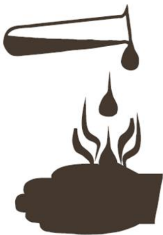
Fig. 10 Corrosive sulfuric acid
